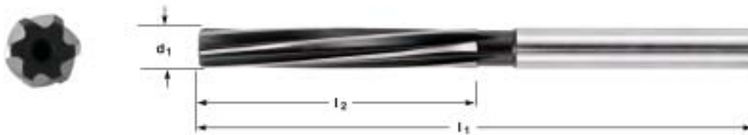
Straight Shank Machine Reamer, Spiral Flute
