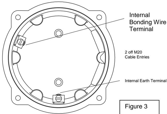
When using the external earth terminal a cable crimp lug must be used. The cable lug should be located between the two M5 stainless steel flat washers. The M5 stainless steel spring washer must be fixed between the outer flat washer and the M5 stainless steel nut to ensure that the cable lug is secured against loosening and twisting.
