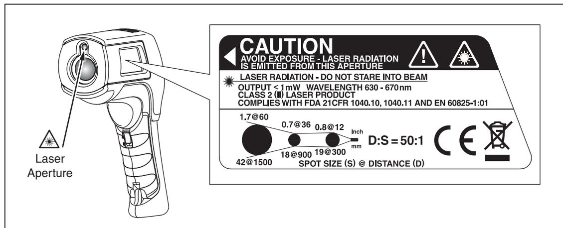
Figure 1. Laser Safety Markings
