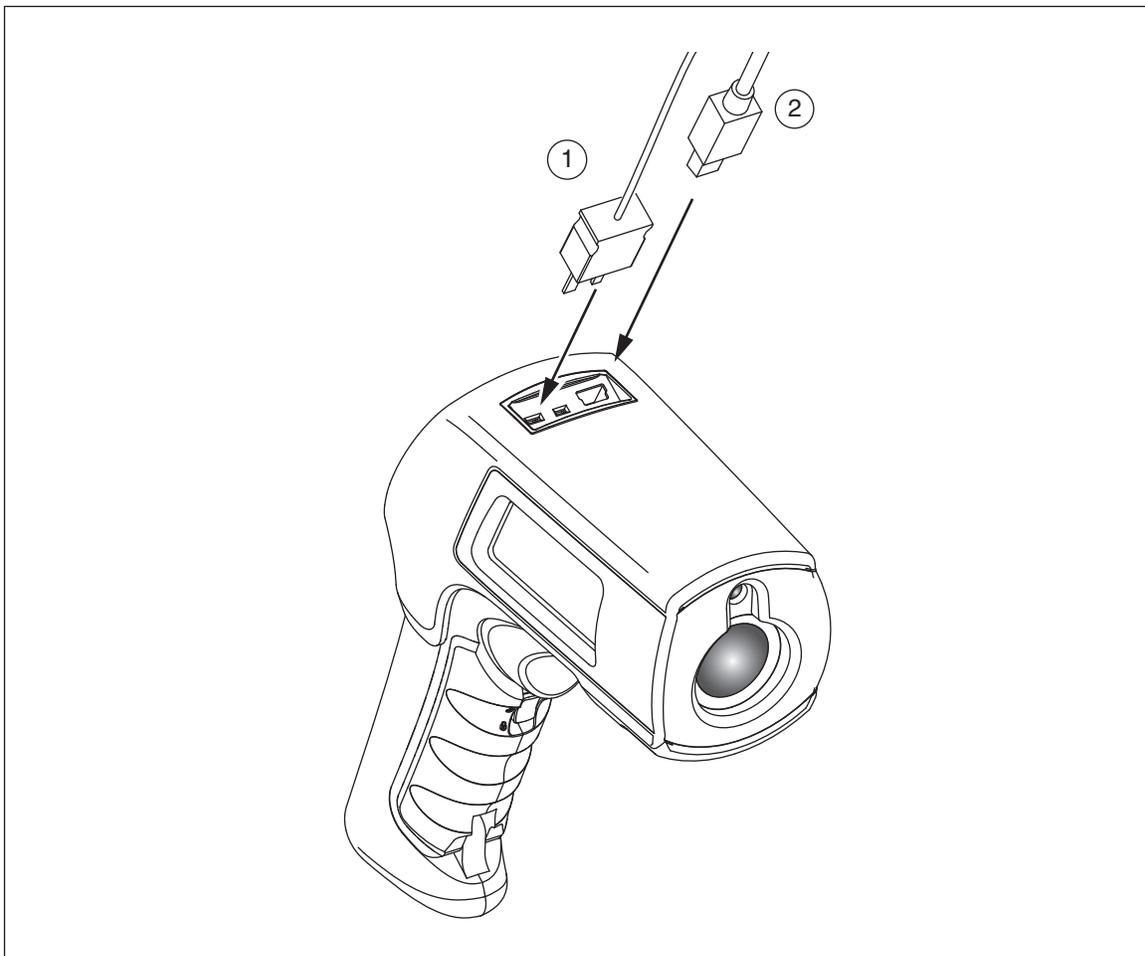
**Figure 7. Thermocouple and USB Connections**
