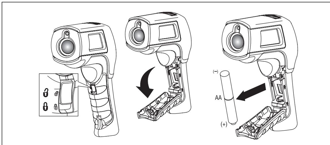
Figure 8. Battery Replacement
