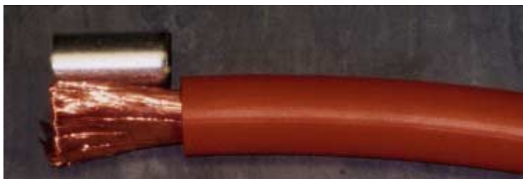
Figure 10. Showing Cable Stripped Alongside Reduction Sleeve
