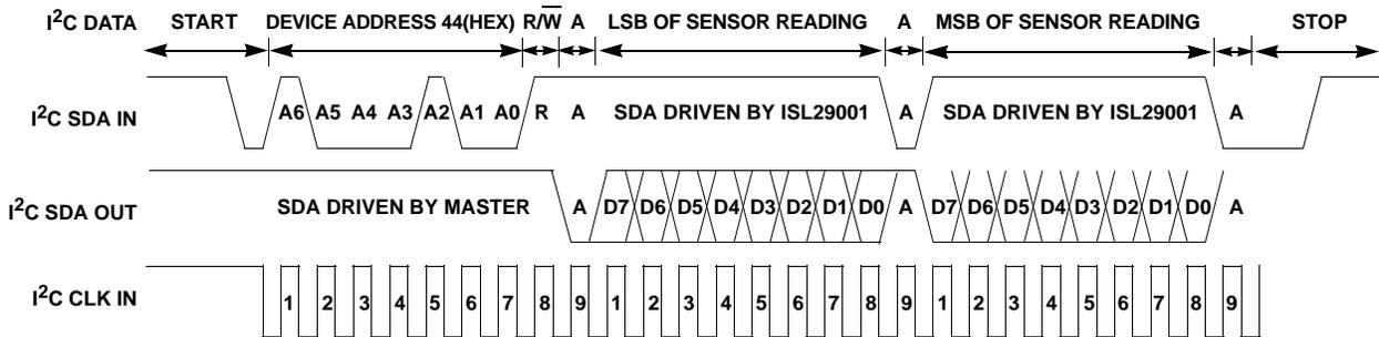
FIGURE 11B. I<sup>2</sup>C READ TIMING DIAGRAM SAMPLE
