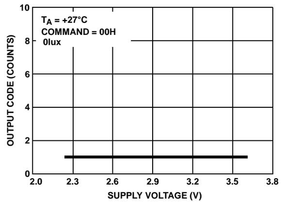
FIGURE 2. OUTPUT CODE FOR 0LUX vs SUPPLY VOLTAGE
