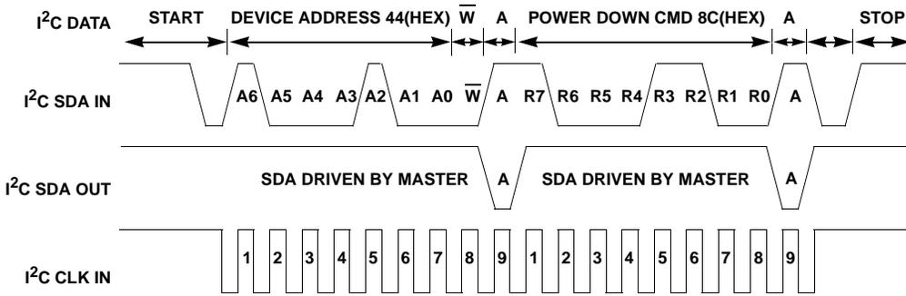
FIGURE 11A. I<sup>2</sup>C WRITE TIMING DIAGRAM SAMPLE
