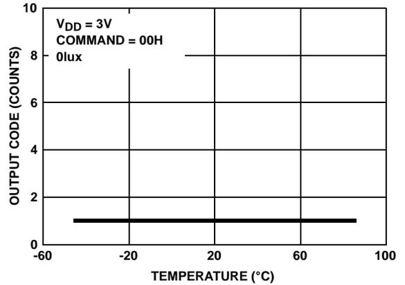
FIGURE 6. OUTPUT CODE FOR 0LUX vs TEMPERATURE
