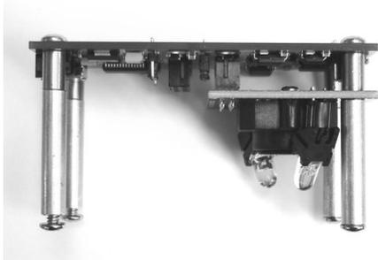
If you are connecting the TCS230-DB to the motherboard via the extension cable (p/n 800-28301), attach the spacers directly to the TCS230-DB using the unused short screws provided with the motherboard.
