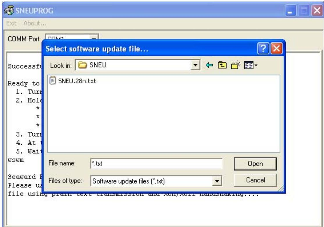
The file will be sent to the tester, this may take several minutes. Information in the text window is for diagnostic purposes, and to satisfy the user that transfer is taking place. During the transfer process the test instrument should beep at a continuous rate. The transfer program will display the following.
