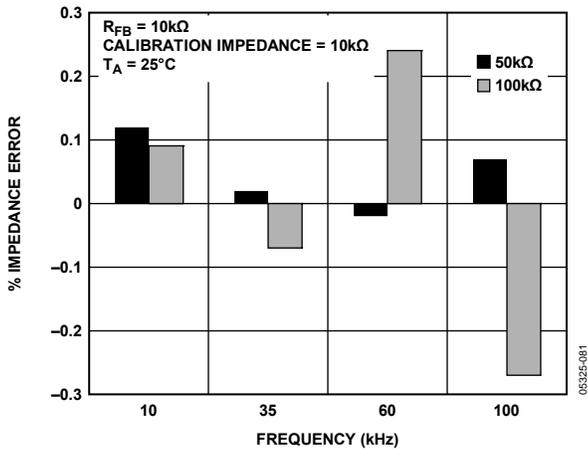
Figure 24. Impedance Range 3 Typical % Impedance Error over Frequency
