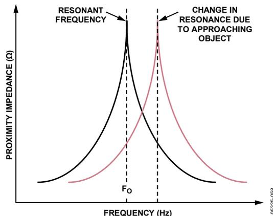
Figure 39. Detecting a Change in Resonant Frequency
