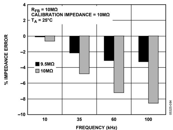
Figure 27. Impedance Range 6 Typical % Impedance Error over Frequency
