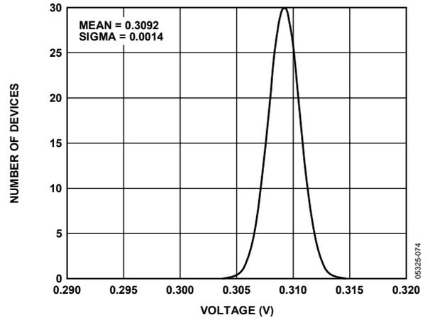
Figure 9. Range 3 DC Bias Distribution, VDD = 3.3 V
