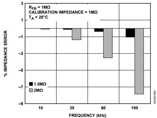
Figure 26. Impedance Range 5 Typical % Impedance Error over Frequency
