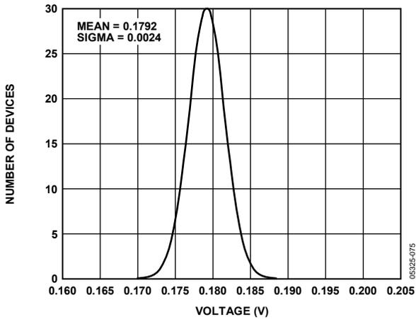
Figure 11. Range 4 DC Bias Distribution, VDD = 3.3 V
