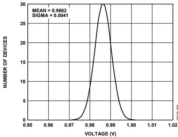
Figure 6. Range 2 Output Excitation Voltage Distribution, VDD = 3.3 V
