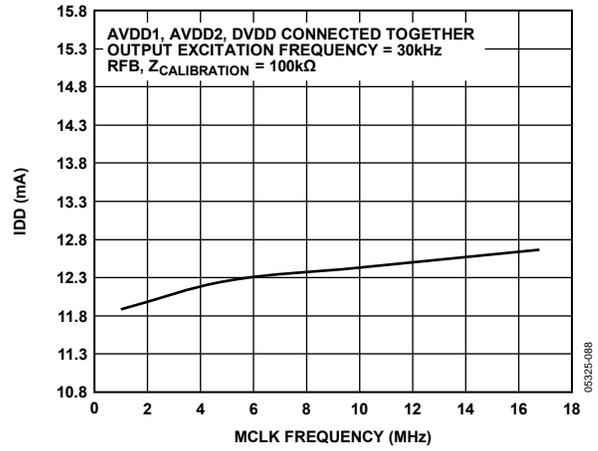
Figure 12. Typical Supply Current (IDD) vs. MCLK Frequency
