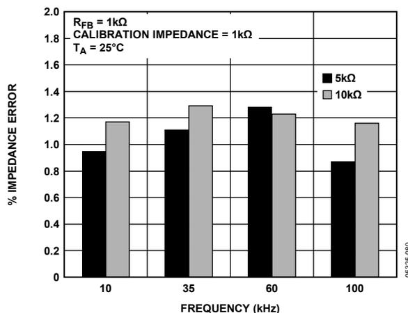
Figure 23. Impedance Range 2 Typical % Impedance Error over Frequency
