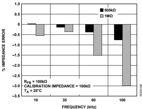
Figure 25. Impedance Range 4 Typical % Impedance Error over Frequency
