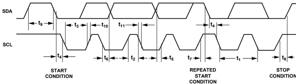
Figure 2. I<sup>2</sup>C Interface Timing Diagram
