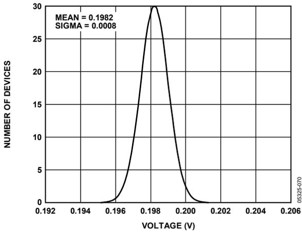
Figure 10. Range 4 Output Excitation Voltage Distribution, VDD = 3.3 V
