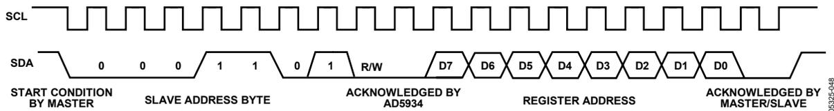
Figure 31. Timing Diagram
