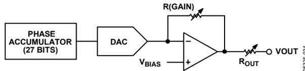
Figure 16. Transmit Stage
