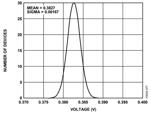
Figure 8. Range 3 Output Excitation Voltage Distribution, VDD = 3.3 V
