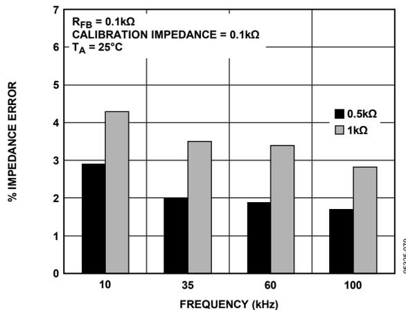
Figure 22. Impedance Range 1 Typical % Impedance Error over Frequency
