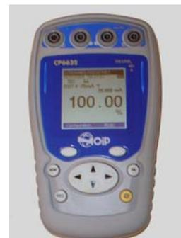
Fully configurable scaling with units: User can also program a scaling in accordance with his sensor or transmitter with unit changing: 4-20mA output signal from a 0-100 bar transmitter will be measured by CP6632 with bar display and reading between 0 and 100 bar.
