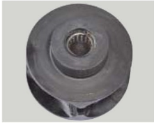
Load chain sheave with needle bearing
