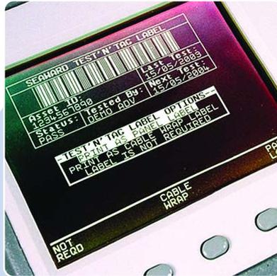
2. On completion of the test routine, choose between panel label and cable wrap label
