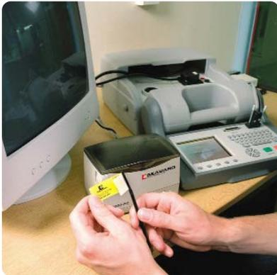
4. Use the peelstick, if needed, to help remove the backing from the panel
