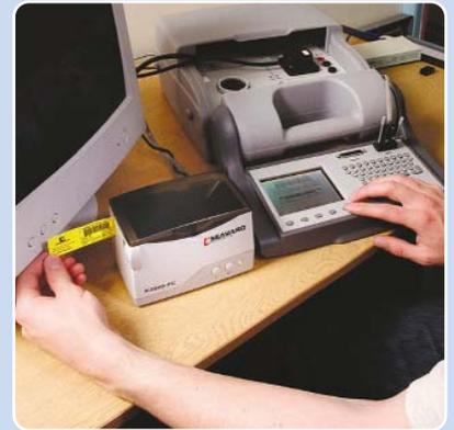
3. Label is printed automatically from the tester
