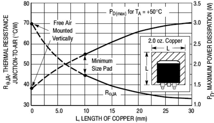
**Figure 1 – D<sup>2</sup>PAK Thermal Resistance and Maximum Power Dissipation vs. P.C.B Copper Length**
