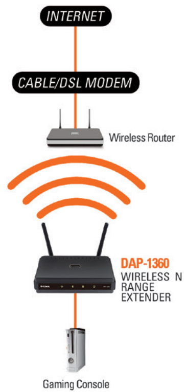
Ethernet-enabled gaming console using the DAP-1360 as a wireless interface to access the Internet
