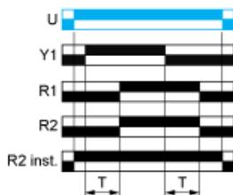
Function Ad : Pulse Delayed Relay with Control Signal
