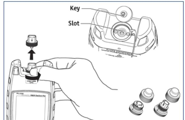
Screw on interchangeable SC adapter. Older models have rectangular latching style adapter.
