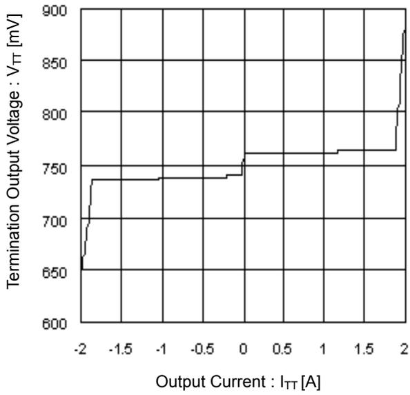
Figure 1. Termination Output Voltage vs Output Current (DDR3)
