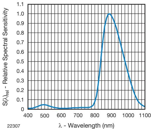
Fig. 10 - Spectral Sensitivity of Proximity PIN Photodiode
