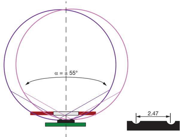
Fig. 8 - Emitter and Detector Angle and Distance
