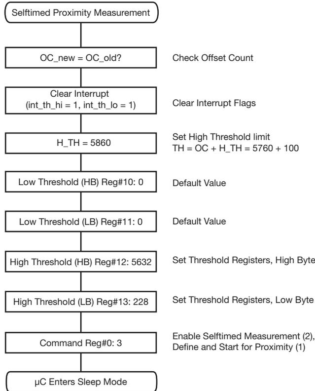
When an object does come close enough to the sensor to generate 100 counts and 4 consecutive measurements occur at or above this level, the interrupt line will go LOW and the interrupt can be read by the microcontroller in register 14 where int\_th\_hi will equal 1.
