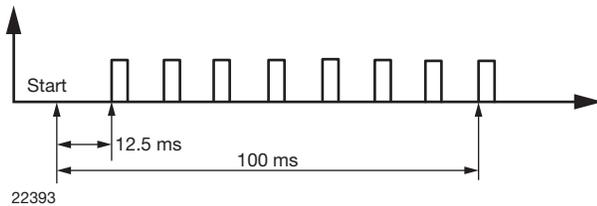
Fig. 17 - Ambient Light Measurement with Averaging = 8
