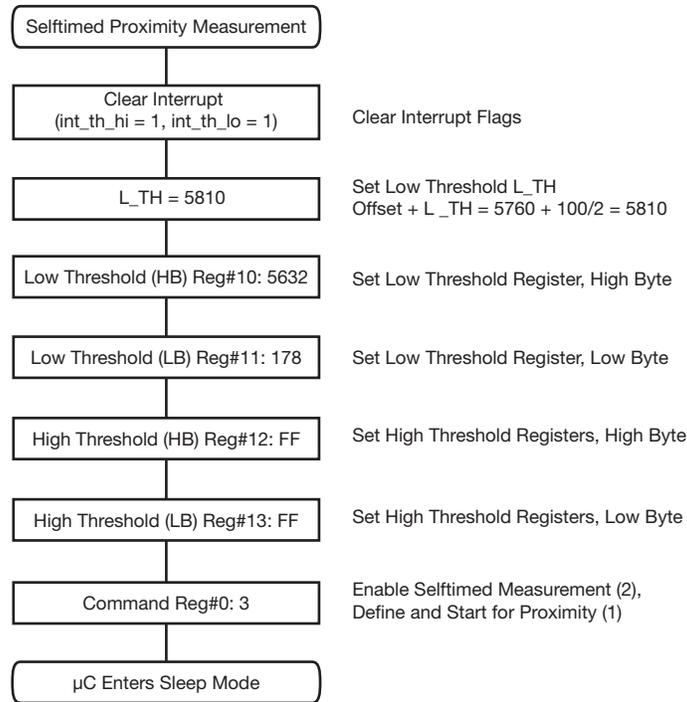
When the object is removed and 4 consecutive measurements occur at or below the lower threshold, the interrupt line will go LOW and the interrupt can be read by the microcontroller in register 14 where int\_th\_lo will equal 1.
