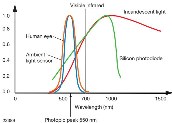
Fig. 14 - Relative Spectral Sensitivity vs. Wavelength
