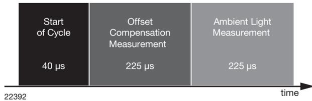
Fig. 16 - Timing Diagram for Individual Measurement Cycle
