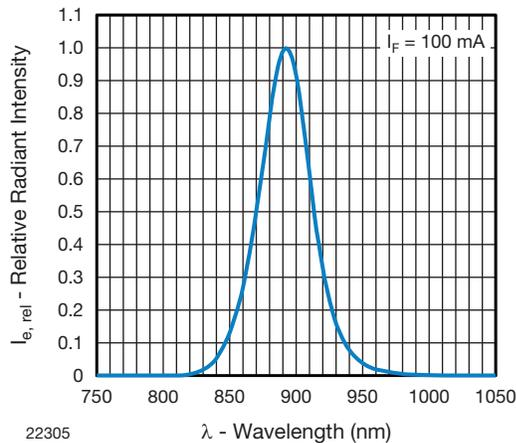
Fig. 4 - Relative Radiant Intensity vs. Wavelength
