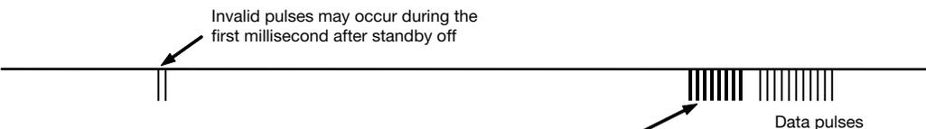
If a signal is received after the latency time (about 1 ms after power up) then the microcontroller will wake up and allow the IR receiver to operate continuously.
