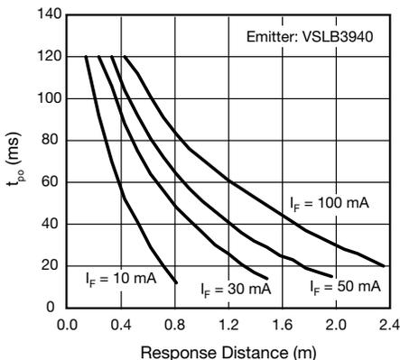
Fig. 7 -  $t_{po}$  vs. Distance Kodak Gray Card Plus 15 %
