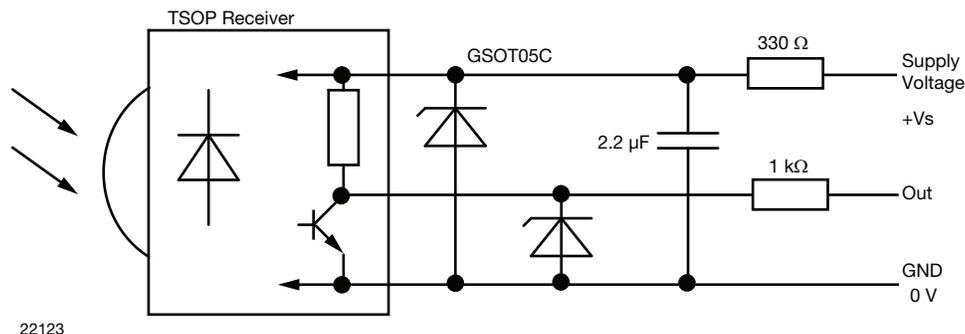
Fig. 2 - Protection Circuit against Over Voltage Spikes
